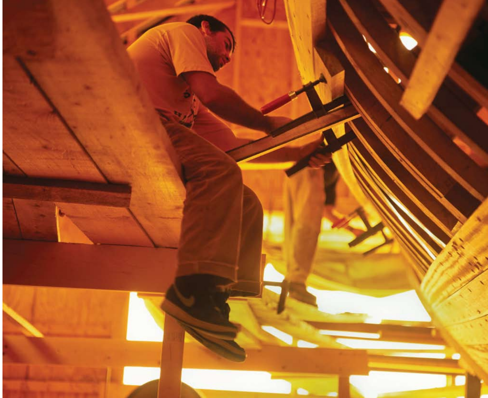
REBECCA'S HULL AFTER RED LEAD (ABOVE); ROSS GANNON, LEFT, AND NAT BENJAMIN SAIL REBECCA (BELOW); CASSON KENNEDY CLAMPS A SILVER BALI PLANK TO A DOUBLE-SAWN FRAME PRIOR TO FASTENING (RIGHT).
