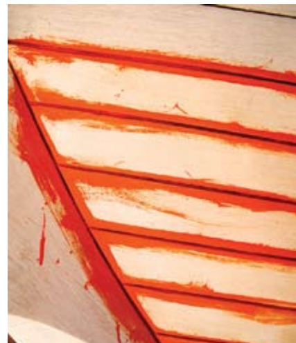
REBECCA'S HULL AFTER RED LEAD (ABOVE); ROSS GANNON, LEFT, AND NAT BENJAMIN SAIL REBECCA (BELOW); CASSON KENNEDY CLAMPS A SILVER BALI PLANK TO A DOUBLE-SAWN FRAME PRIOR TO FASTENING (RIGHT).
